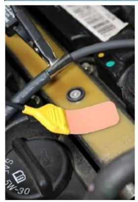
A capacitive probe should have a ground clamp as part of the test leads. This creates an easier path to ground for the thousands of volts generated by the coil. If the probe or clamp is not grounded, the voltage could damage the internal circuitry of the scope. Most scopes have a limit around 200 volts, and most ignition systems can generate more than a 4,000 volts.
