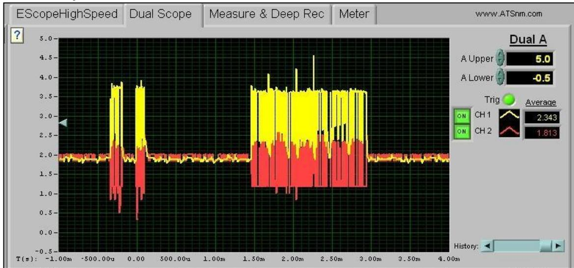
The next capture shows the GMLAN activity with the Scan Tool communicating with the CAN modules. Note that the bias is now closer to 3.5 Volts. You won't see these results for other manufacturers, so it's important to know that it is normal for *some* GM applications.
