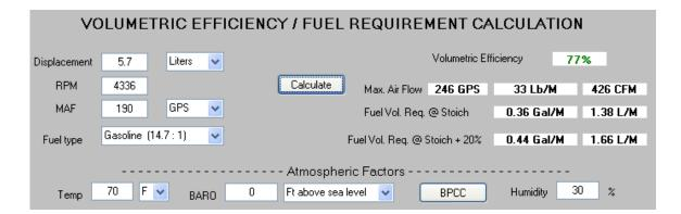
The previous example illustrates a VE entry for a 5.7 Liter GM truck that was driven at wide open throttle and had its peak recorded RPM and MAF values entered.
