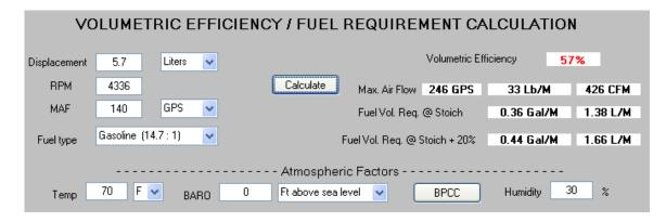
This example shows how the same test drive can confirm a VE issue based on the entered data. In this case the problem was an air metering issue, specifically the MAF sensor.
