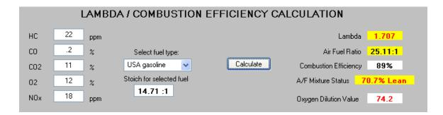
In this final example we can see a big red (or rather yellow) flag. An Oxygen dilution value of less than 75 triggers the Lambda related outputs to be highlighted in yellow. This is because the values reported in these boxes are probably incorrect due to the presence of excess Oxygen. If this situation arises, air injection should be disabled and exhaust systems should be checked for leaks to insure the accuracy of these calculations.
