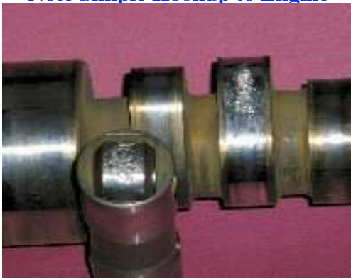
Photo of parts replaced showing cam and roller damage.
