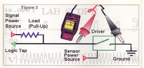
Because this is a sensor circuit, and not an actuator circuit, there is no need for high current flow. So the pull-up resistor usually has a high resistance value. One source reports values of more than 500 ohms, but usually less than 1 K ohms for the pull-up resistor.
