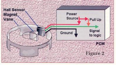
the output. It simply tells the transistor when to switch. The transistor is said to have an *open collector output*. This means that it is no more then a simple switch to ground. It is the signal power source that supplies the voltage to the transistor to create the signal.
