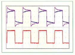
Here are some examples of how probe compensation can effect waveforms. This adjustment should be performed periodically.
