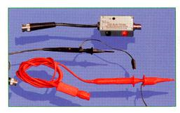
Three different 10:1 probes. The top probe was designed for automotive use. Two probe taps in the side allows you to connect a second set of test leads. The center probe is designed for electronic applications and can be rather fragile, especially near heat. The lower probe is a Fluke product, also designed for automotive use.
