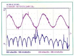
It is common to see noise, especially when the scope is adjusted to low voltage and time per division settings. The spikes in these signals represent noise in the ignition system, and have no other significance.
