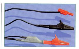
Here are some examples of shielded leads. The top lead utilizes a stacking sheathed banana plug, and is supplied with the Edge PAC scope. The lower lead set is supplied with the Fluke 98, and features a removable ground lead that attaches at the gray connector.
