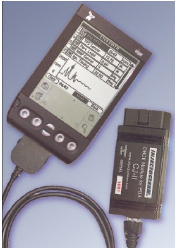
This PDA is connected to an OBD II interface module. OBD II data can be quickly retrieved with this pocket-size tool.
