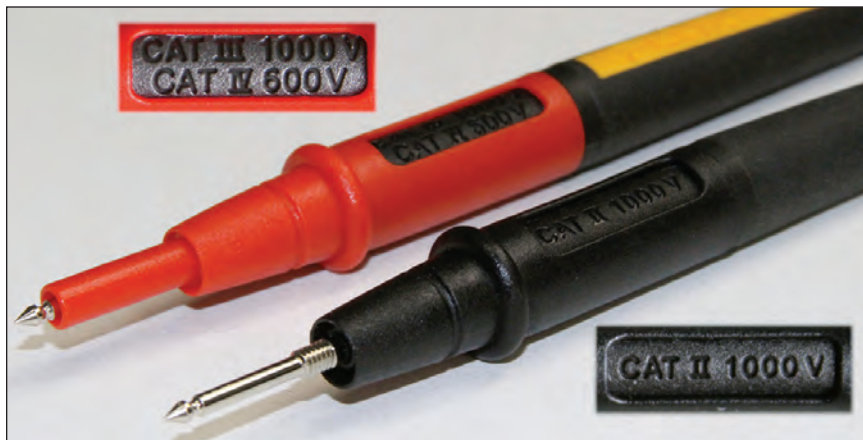
The red Fluke test probe in this photo can be twisted to lock it into either CAT III 1000V or CAT IV 600V configuration. The black probe has a single CAT II 1000V rating.
