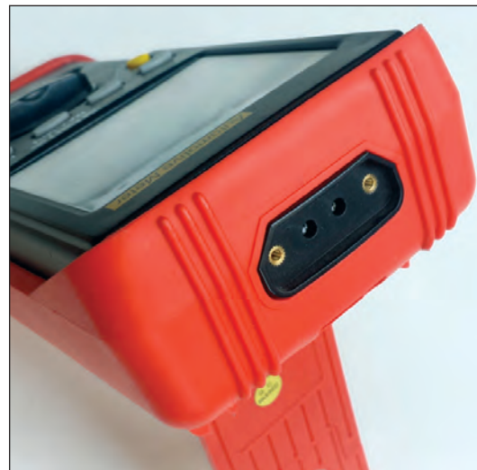
An optically isolated USB charging port on this scope completely separates signal grounds from earth ground. This makes it safer and more accurate to use than a scope that features shared grounds.
