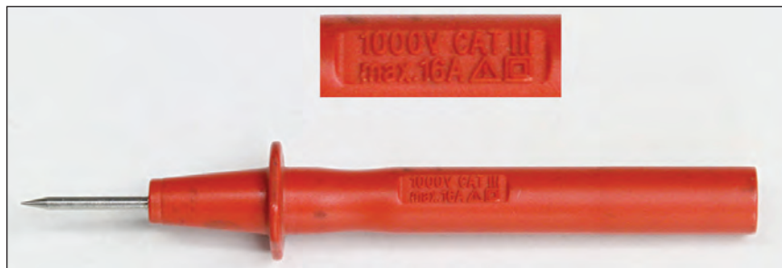
Markings on scope test probes should provide an indication of their operating limitations. Use reputable suppliers, as some probes (like this one) include inaccurate rating information.
