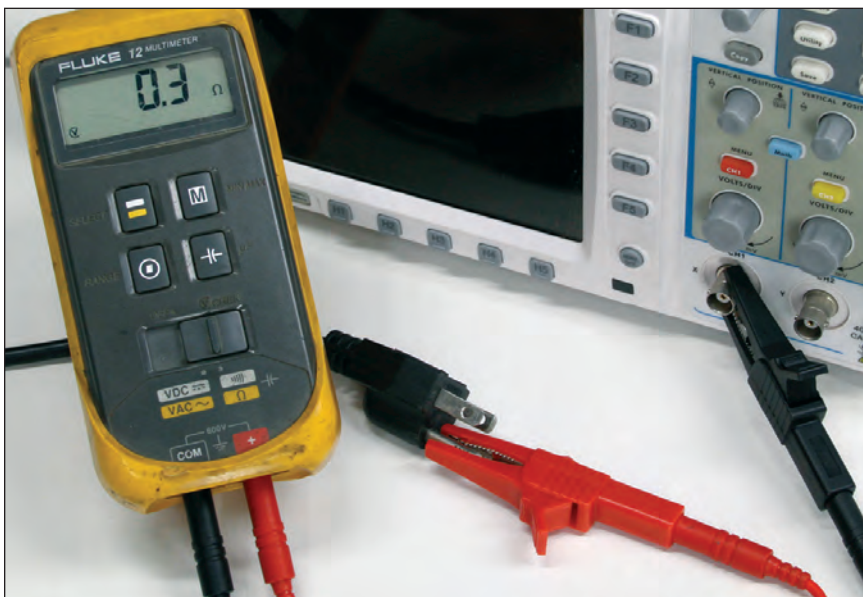
This simple test will help you determine whether a scope's signal grounds are connected to earth ground. The DMM's low resistance reading indicates a direct connection between the two.
