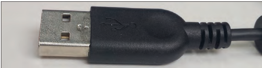
The metal shell of the USB connector connects the instrument ground to a PC. Scopes using this type of connection share common signal and earth grounds.
