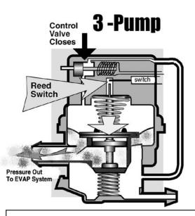
The LDP sense switch circuit is the only EVAP monitor input to the PCM. Since the switch is normally closed, look for battery voltage at the PCM switch pin KOEO. The switch circuit voltage drops to zero when vacuum pulls the pump diaphragm upwards far enough to open the switch.
