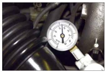
On a normal engine, idle vacuum should be steady between 17 and 21 in. of vacuum. Once again, larger engines that are in good shape will tend to produce higher vacuum readings at idle than smaller engines with fewer cylinders.
