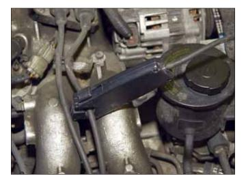
nal. An oscilloscope is a very useful tool for testing electronic signals. A transducer can take a certain condition and convert it into an electronic signal. For example, the vacuum pulse from an engine can be converted in this way. Using a transducer to convert a vacuum pulse into an electrical signal, then synchronizing it with the ignition produces a very useful scope pattern.
