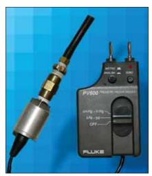
This Fluke transducer can read vacuum or pressure and can be used with a scope or a DSO. DSO use requires an adapter to convert the transducer's banana plugs to the scope's BNC connector.
