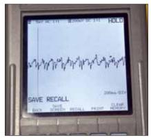
Think of a vacuum waveform as an inverted signal. An increase in pressure drives the signal lower. A conversion factor is necessary to translate the voltage levels shown in the vacuum waveform to actual vacuum readings. This conversion factor is specific to individual transducer types.
