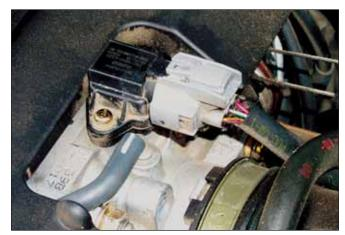
The MAP sensor can also be used to collect vacuum readings, as long as you've figured out the conversion factor. Remember, vacuum is really pressure that's less than atmospheric pressure. The MAP sensor measures manifold absolute pressure.
