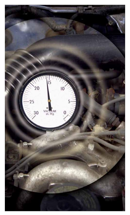
However, if we move the throttle plates open, the vacuum will decrease—as long as engine speed remains constant. It's important to understand this basic concept before moving further.
