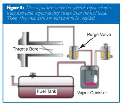
The *power-up test* is a passive test designed to detect restrictions or blockages in the vent path. The test runs when the vent valve is open, the purge valve is closed, the engine is cold and the ignition key is in the RUN position with the engine OFF. The test only runs when all of the enable criteria are met. For example: the fuel level must be somewhere between 15 and 85%. Under normal conditions, the fuel tank pressure sensor should not indicate excessive vacuum during this test.
