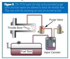
While a vacuum is still present in the fuel tank, the vent and purge valves are commanded closed to seal the system. The PCM then monitors the fuel tank pressure sensor to determine the rate of vacuum loss (decay). If the decay rate is too fast, the PCM will store a small leak DTC. Early systems are calibrated to detect leaks as small as 0.040inch (1 mm), while newer systems can detect leaks half that size (0.020-inch or .5 mm).
