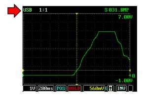
**NOTE:** The uScope must be on and be displaying the waveform grid. (Do not press the <DOWN ARROW> while powering up.)
