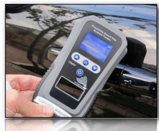
OPERATE THE PROXIMITY SYSTEM BY TOUCHING THE SENSOR, BUTTON OR OPENING THE DOOR.
