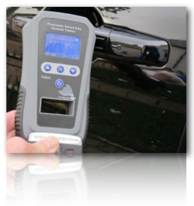
IN OSCILLOSCOPE MODE THE SIGNAL LEVEL OF THE SMART/PROXIMITY KEY CAN BE VIEWED AND COMPARED.
