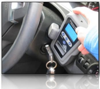
SELECT THE COIL ANTENNA TEST FROM THE MAIN MENU.
