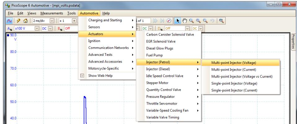
This menu displays a selection of the common measurements that can be taken using the Automotive Kit. When you select one of the measurement options from the menu, PicoScope will automatically:
